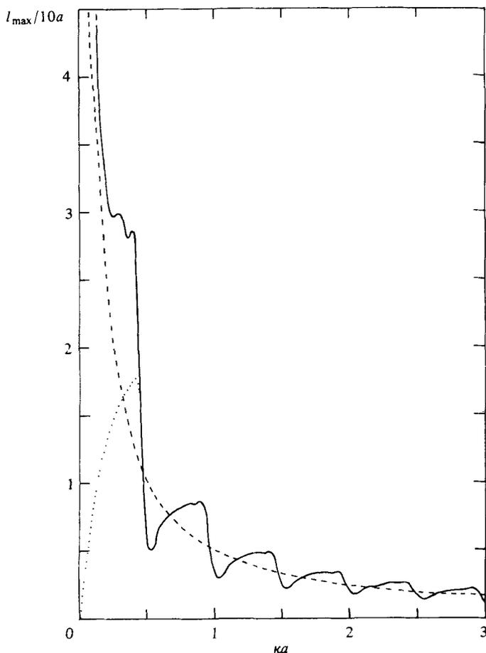
FIGURE 10. Variation of the non-dimensional maximum absorption length  $l_{\max}/10a$  with frequency  $\kappa a$  for an optimally tuned row of five equally spaced semi-immersed spheres in beam seas. The spacing between the bodies is fixed at  $d = 12.5a$ . —,  $l_{\max}/10a$  for unconstrained optimal motion;  $\dots$ ,  $l_{\text{abs}}/10a$  for constrained motion, maximum body displacement  $< 3$  times incident wave amplitude; - - -, mean gain factor  $q = 1$ .
