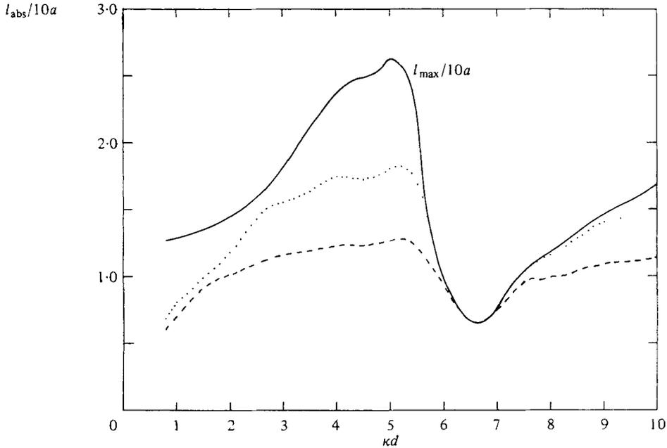
FIGURE 6. Variation of the non-dimensional absorption length  $l_{\text{abs}}/10a$  with body spacing for the single row of semi-immersed spheres in beam seas. —, optimal unconstrained motion; . . ., constrained motion, maximum body displacement  $<$  three times incident wave amplitude; - - - constrained motion, maximum body displacement  $<$  twice incident wave amplitude.
