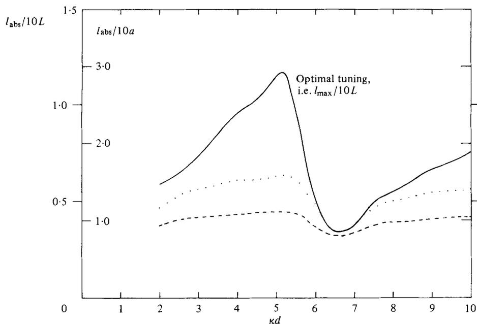
FIGURE 14. Variation of the non-dimensional absorption length  $l_{\text{abs}}/10L$  with body spacing for the single row of five thin ships in beam seas. —, optimal unconstrained motion (i.e.  $l_{\text{max}}/10L$ );  $\dots$ , constrained motion, maximum body displacement  $<$  three times incident wave amplitude;  $---$ , constrained motion, maximum body displacement  $<$  twice incident wave amplitude. The scale  $l_{\text{abs}}/10a$  is also shown to enable comparison with figure 6.
