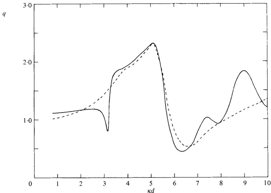
FIGURE 7. Variation of the mean gain factor  $q$  with body spacing for an optimally tuned double row and an optimally tuned single row of semi-immersed spheres in beam seas. The spacing between the rows of the double row is equal to the spacing between adjacent members of each row, i.e.  $c = d$ . —, double row; ---, single row.
