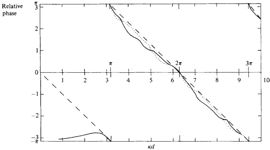
FIGURE 5. Variation of the relative phase, i.e. the phase difference between two adjacent bodies, with the body spacing for the optimally tuned single row of semi-immersed spheres in head seas. —, the relative phase of the (first and second) and (fourth and fifth) bodies; . . ., the (second and third) and (third and fourth) bodies; - - -, a constant phase difference of  $-\kappa d$ .
